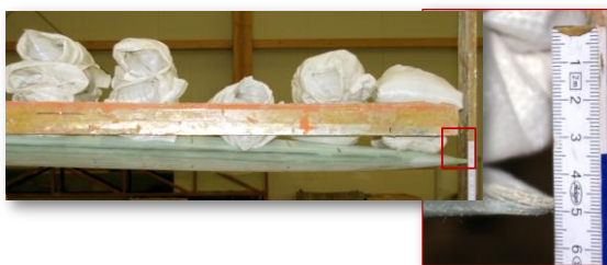
Figure 7 Static load test of the prototype tip extension in the laboratory. The right side shows the deflection at maximum load.
